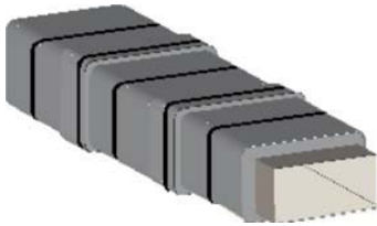
Single Layer System with 76mm (3") overlap Installation
