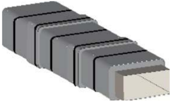
Single Layer System with 76mm (3") overlap Installation
